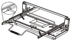
For each side, support the side rail with one hand and with the other hand lift the frame up and out of the side clips.
